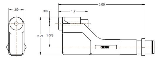
The H856-6MB Offset Pulling Head installs 3/16" diameter (-06) MAXIBOLT®.
