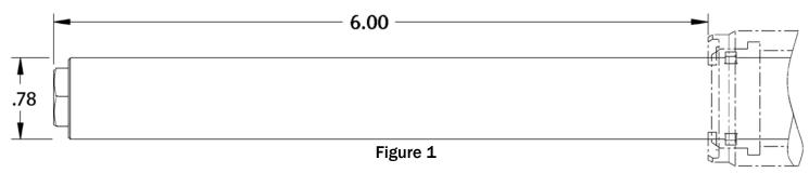
DIMENSIONAL DATA (all measurements in Inches, see figure 1) Pulling Head Weight: 4.2 Lbs (1.9 kg)
