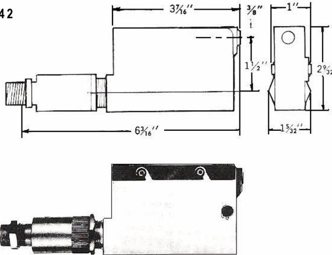
These heads fit directly on Cherry® Riveters G-11, G-15 and G-36. They also fit on G684 and G784 riveters with appropriate adapters (see page 4)
