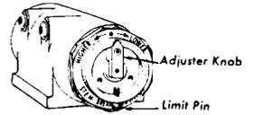
Tool will now install Cherrylock rivets up to 1/2" grip length. Before using a straight H681 pulling head again, the riveter must be readjusted using a 680A159 setting gage. Reverse steps 1 & 2 above and adjust riveter until gage point is flush with tool head.
