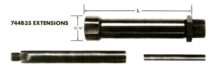
These extensions, by using one or any combination, will help reach into many restricted installation areas by increasing the overall length of the pulling head. They fit directly onto the G-744 CherryMAX® power riveter and will accept any of the 1/4" CherryMAX® pulling heads.
